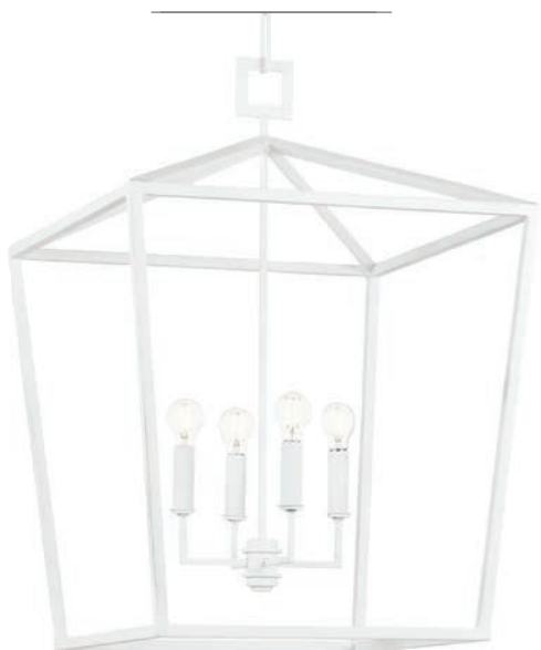
9000-0977 DENISON GRANDE WHITE LANTERN H: 48" W: 32" D: 32" Adjustable: 57" to 148" Canopy: Round, H: 1" Dia: 6" Chain (Extra): 8' (1) (0100-0070) Materials: Wrought Iron Finish: Gesso White 5 Lights Bulb/Socket: A Standard Bulb/E26
